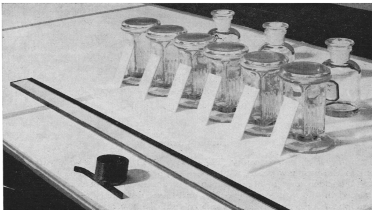
Fig. 1. Applicator and developing jars for microchromatoplates.
